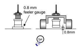
3 Set the sensor gap to 0% and press the "Set" button on the converter.
