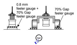
17 Set the sensor gap to 70% and press the "Set" button on the converter. \*12
