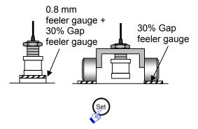
9 Set the sensor gap to 30% and press the "Set" button on the converter. \*8
