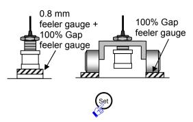
Set the sensor gap to 100% and press the "Set" button on the converter. \*15
