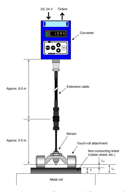
L<sub>1</sub>: Distance to the metal roll from the sensor tip surface
