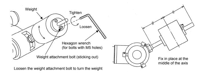
Loosen the weight angle adjustment nut to change the weight angle and make a coarse adjustment to the pressure applied to the roller. (Placing the weight in an upright position increases the roller pressure).
