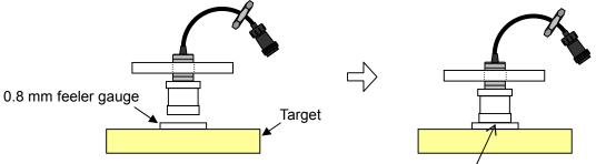
Turn the sensor body and let the sensor tip touch the 0.8 mm feeler gauge. Be careful not to damage the sensor tip.
