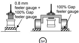
Set the sensor gap to 100% and press the "Set" button on the converter. \*1
