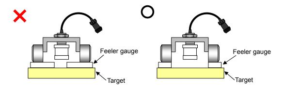
• When making an adjustment by directly placing the feeler gauge on the sensor
