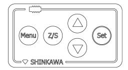
While pressing and holding the [Menu] button, [Z/S] button (press) -> [ $\triangle$ ] button (press) -> [ $\nabla$ ] button (press) -> [Set] button (long press)
