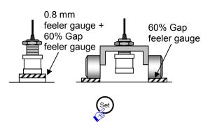
9 Set the sensor gap to 60% and press the "Set" button on the converter. \*3
