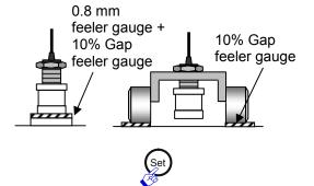
5 Set the sensor gap to 10% and press the "Set" button on the converter. \*6
