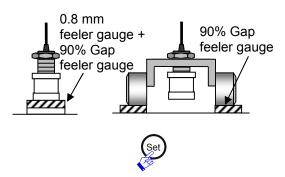
21 Set the sensor gap to 90% and press the "Set" button on the converter. \*14
