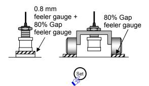
11 Set the sensor gap to 80% and press the "Set" button on the converter. \*4
