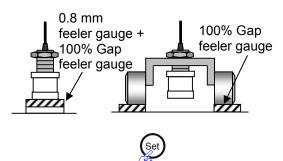
7 Set the sensor gap to 100% and press the "Set" button on the converter. \*3
