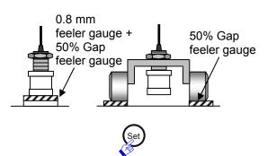
13 Set the sensor gap to 50% and press the "Set" button on the converter. \*10
