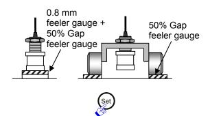
5 Set the sensor gap to 50% and press the "Set" button on the converter. \*2
