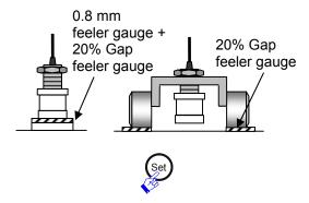
7 Set the sensor gap to 20% and press the "Set" button on the converter. \*7
