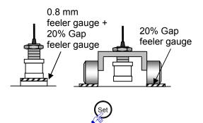
5 Set the sensor gap to 20% and press the "Set" button on the converter. \*1
