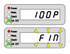
The seven-segment LED display will show "100P" (1.5 seconds), and then flash indicate "FIN".
