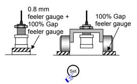
13 Set the sensor gap to 100% and press the "Set" button on the converter. \*5
