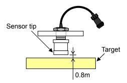
**Point** Depending on the usage environment of the sensor, tighten the jam nut with a torque of 176 Nm as a standard.
