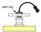
**Point** Depending on the usage environment of the sensor, tighten the jam nut with a torque of 176 Nm as a standard.
