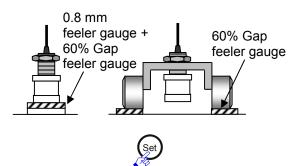
15 Set the sensor gap to 60% and press the "Set" button on the converter. \*11
