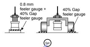
7 Set the sensor gap to 40% and press the "Set" button on the converter. \*2
