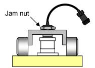
**Point** Depending on the usage environment of the sensor, tighten the jam nut with a torque of 176 Nm as a standard.
