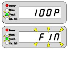
The seven-segment LED display will show "100P" (1.5 seconds), and then flash indicate "FIN".
