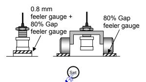
19 Set the sensor gap to 80% and press the "Set" button on the converter. \*13
