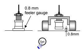
Set the sensor gap to 0% and press the "Set" button on the converter.
