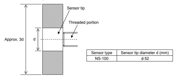
You need to be careful if you are using a jig other than the special attachment since there are cases where performance is decreased if conductors such as metals are present in the portion indicated in the diagram above.
