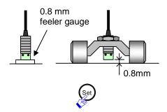
3 Set the sensor gap to 0% and press the "Set" button on the converter.
