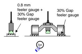
9 Set the sensor gap to 30% and press the "Set" button on the converter. \*8
