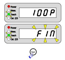
14 The seven-segment LED display will show "100P" (1.5 seconds), and then flash indicate "FIN".
