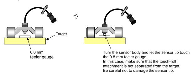
4 Fix the sensor in place by tightening the jam nut.
