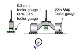
9 Set the sensor gap to 60% and press the "Set" button on the converter. \*3
