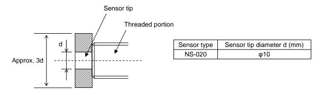
You need to be careful if you are using a jig other than the special attachment since there are cases where performance is decreased if conductors such as metals are present in the portion indicated in the diagram above.
