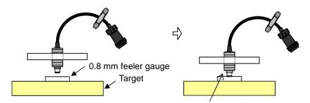
Turn the sensor body and let the sensor tip touch the 0.8 mm feeler gauge.
