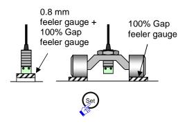
5 Set the sensor gap to 100% and press the "Set" button on the converter.
