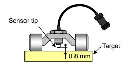
Lift the touch-roll attachment and attach the sensor cover to the sensor tip.
