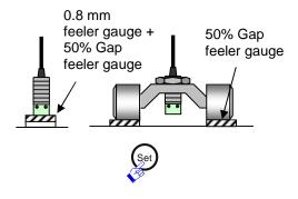
Set the sensor gap to 50% and press the "Set" button on the converter. \*10
