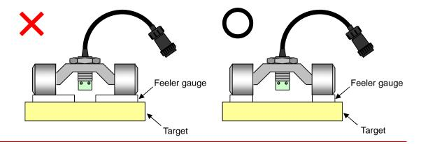
• When making an adjustment by directly placing the feeler gauge on the sensor
