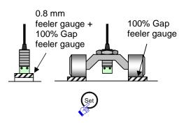
13 Set the sensor gap to 100% and press the "Set" button on the converter. \*5
