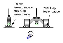
17 Set the sensor gap to 70% and press the "Set" button on the converter. 12
