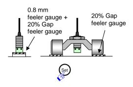
5 Set the sensor gap to 20% and press the "Set" button on the converter. \*1
