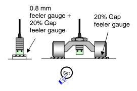
7 Set the sensor gap to 20% and press the "Set" button on the converter. <sup>17</sup>
