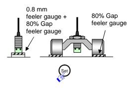
11 Set the sensor gap to 80% and press the "Set" button on the converter. \*4
