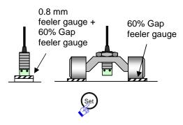
15 Set the sensor gap to 60% and press the "Set" button on the converter. \*11
