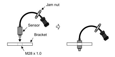
Insert a 0.8 mm feeler gauge between the sensor tip and the target and adjust the position of the sensor.
