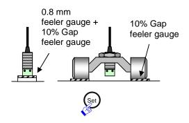
5 Set the sensor gap to 10% and press the "Set" button on the converter. \*6
