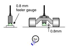
3 Set the sensor gap to 0% and press the "Set" button on the converter.
