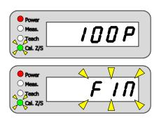
8 The seven-segment LED display will show "100P" (1.5 seconds), and then flash indicate "FIN".
