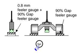
2 1 Set the sensor gap to 90% and press the "Set" button on the converter. \*14
