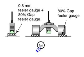
Set the sensor gap to 80% and press the "Set" button on the converter. \*13
