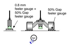
5 Set the sensor gap to 50% and press the "Set" button on the converter. \*2
