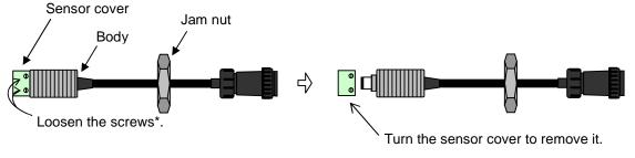
\* The sensor cover can be removed by lightly loosening it.
