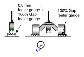
23 Set the sensor gap to 100% and press the "Set" button on the converter. \*15
