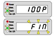
The seven-segment LED display will show "100P" (1.5 seconds), and then flash indicate "FIN".
