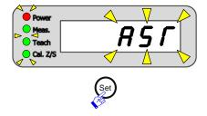
All LEDs that display status will flash, and the seven-segment LED display will flash indicate "RST".
