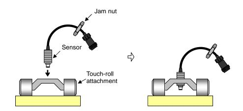
Insert a 0.8 mm feeler gauge between the sensor tip and the target and adjust the position of the sensor.
