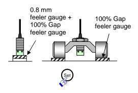
7 Set the sensor gap to 100% and press the "Set" button on the converter. \*3
