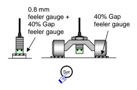
7 Set the sensor gap to 40% and press the "Set" button on the converter. \*2
